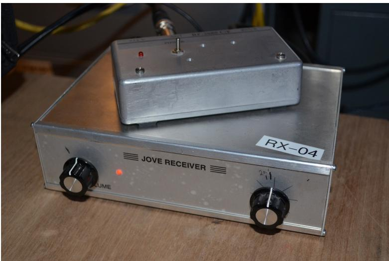
The Radio Jove is a fairly low powered box. The box on top is a 25 K (kelvin) noise source when turned on and becomes a band-pass filter to reduce SW broadcast interference. I used a HP signal generator to verify the settings and the weak signal response. I could see a signal as low as a 0.1 microvolt. To avoid power noise, I also use a well-regulated 12 volt DC wall-wart power supply to drive both units.
